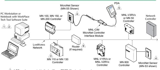
√1\ A PC can be connected to the LonWorks TP/FT-10 network, either directly or through the LonWorks network jack of a LONWORKS controller or MN-Sx wall sensor. The PC must have an Echelon LonTalk Adapter card.
