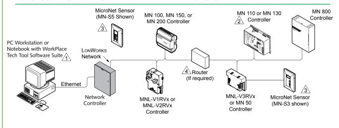
Programming any of the MicroNet LON controllers, or the TAC I/A Series MN 800 controller, requires WorkPlace Tech Tool (WP Tech).
